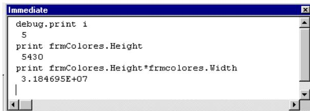
Figura 2.14. Ventana *Immediate*.
